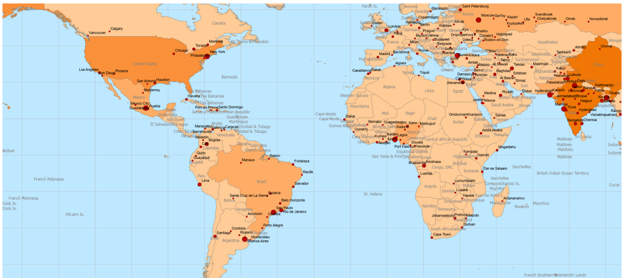
Ch 2— country and city names can be seen after zooming in from Full Extent. Country names are at a lower transparency than cities. City population centers can also be seen, as well as country population (graduated colors).
